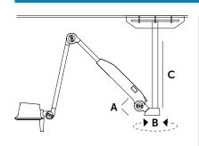
$A = 90^{\circ} (\pm 45^{\circ}) B = 360^{\circ}$ **C** = FROM 250 mm TO 1.100 mm
